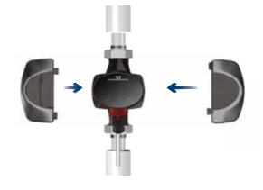
Fig. 44 Insulating shells
