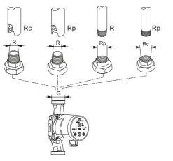
Fig. 43 G-threads and R-threads
