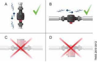
Fig. 2 Control box positions
