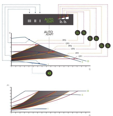
Fig. 36 Performance curves in relation to pump setting
