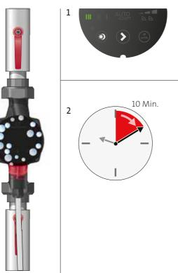
Fig. 13 Venting the pump
