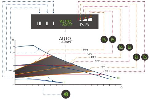
Fig. 29 Pump setting in relation to pump performance
