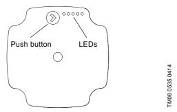
Fig. 46 User interface with one push button and five LEDs
