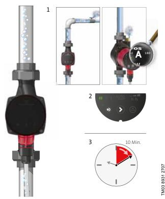
Fig. 14 Venting of the heating system
