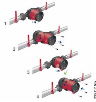
**Fig. 5** Changing the control box position You can turn the control box in steps of 90 °.
