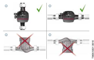
Fig. 7 Position of the ALPHA SOLAR control box
