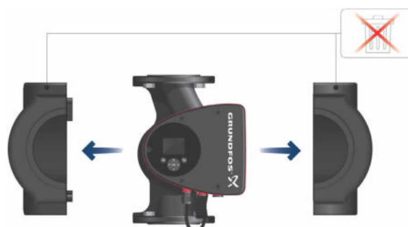
Fig. 3 Fitting insulating shells to the pump
