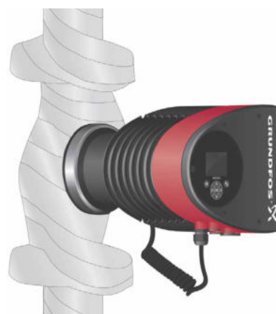
Fig. 4 Insulation of pump housing and pipework
