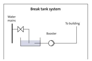
It is recommendable to install a water shortage detection on the suction side the booster. By direct boosting systems a pressure switch can be used – in case of a break tank system, a level switch in the tank will be the best solution.
