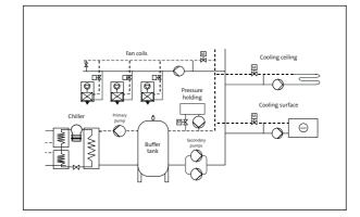
If the chiller is not controlled by this return temperature, we recommend the use of variable speed pumps mounted in parallel up to a maximum of 4 pumps.
