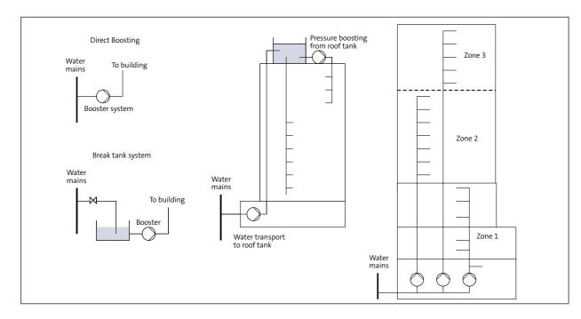
Pressure boosting large buildings is necessary whenever the public water supply is inadequate, either because of too low pressure or because of too low flow to supply the building during peak consumption. The objective is to ensure a constant pressure throughout the building.
