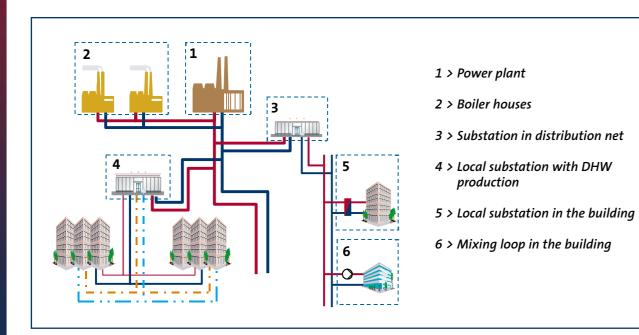
District heating describes a water-based heating system where there is a considerable distance between the place the heat is generated (power plant) and the place the heat is used (the building).
