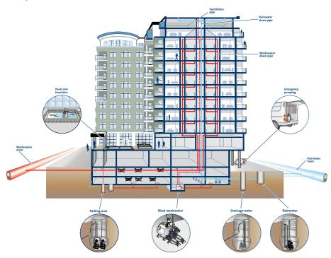
Wastewater in building, especially in commercial building need to be collected and discharged to the main sewer systems outside the building when sanitary applicances, cantines, backwashfilter from swimmimg pools, drainage, deep-level garages etc. are located in the basements below the sewer system outside. The must to effluent these sections of the buildings is beyond dispute.
